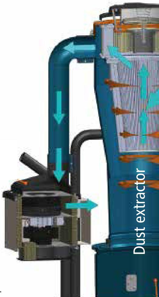
1. Large particles are separated dynamically in the **Cyclone**.
