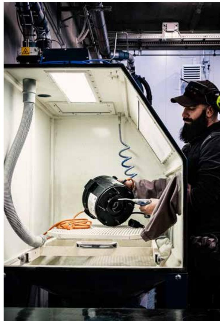
Compressed air connection and blow gun nozzle.
