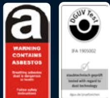
**Warning label – Asbestos.** This device is H-classified and third party certified by a notified body according to EN 60335-2-69, Annex AA and TRGS 519.
