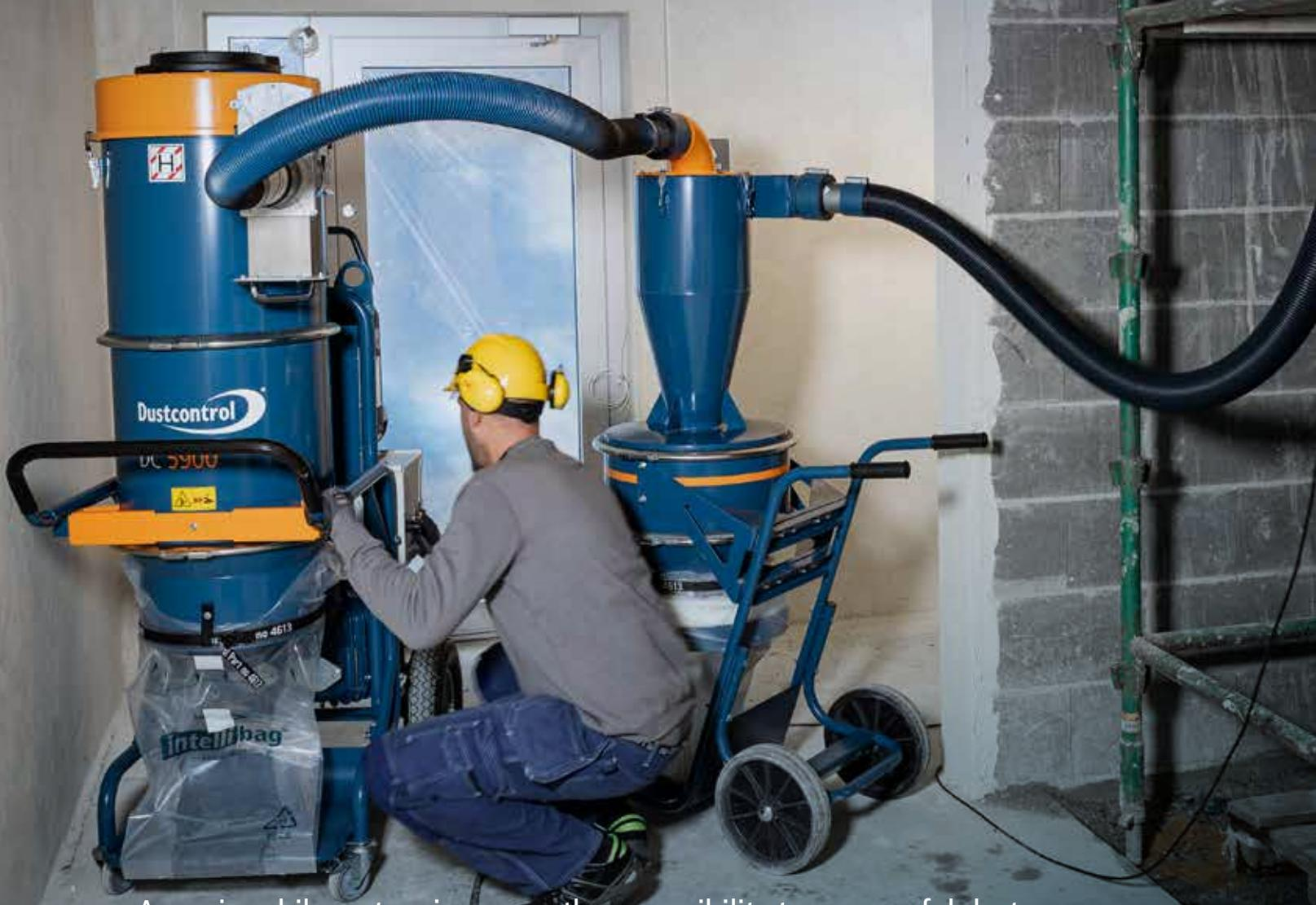
A semi-mobile system increases the accessibility to a powerful dust extractor on each floor. Instead of moving several small and large dust extractors around, multiple users can simultaneously connect their machines or power tools via a hose to a connection point.
